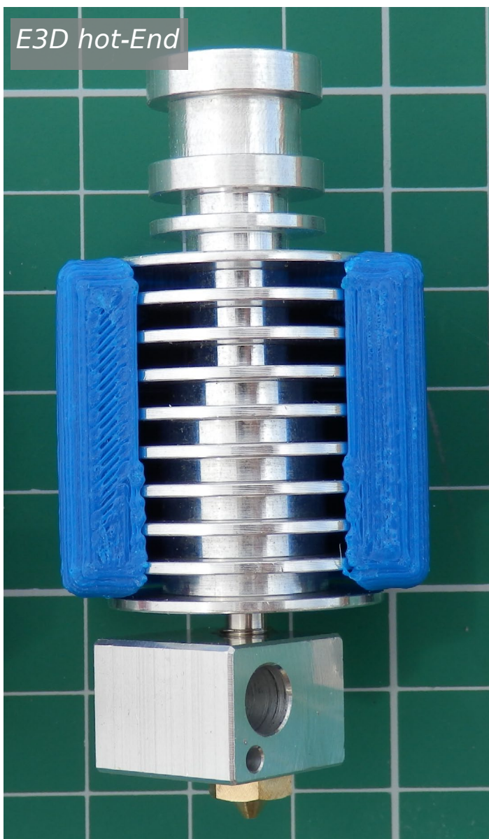
Cube almost finished printed PLA -E3D Hot-End -190deg -65mm/sec
