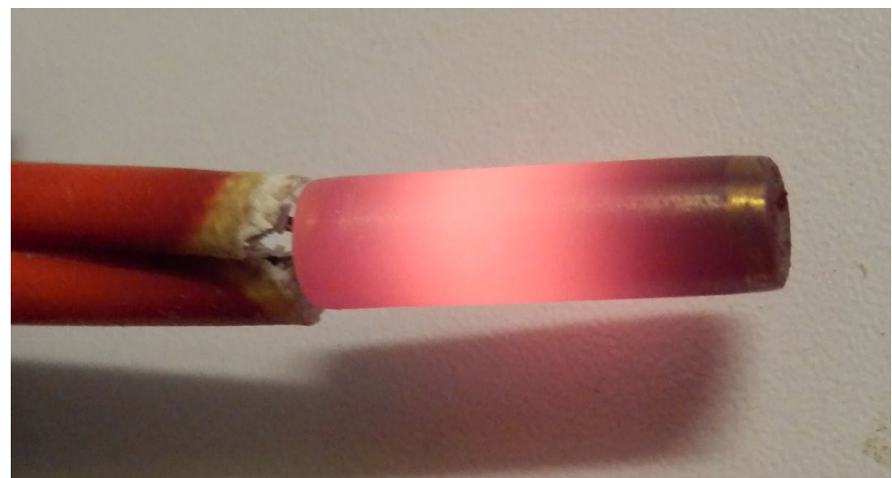
Running a cartridge heater at 12v, this is current limited 2.7A by my power supply, still glowing red-hot and burning the insulation.
