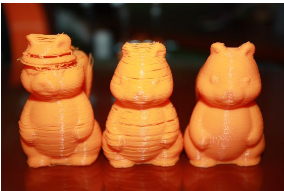
Left: A filament drive problem caused the print failure. Middle: Printed without tweaking the bowden extruder. Right: With bowden modifications.
