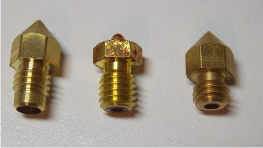
Similar but different - Left is a PICO nozzle, E3D in the middle and QUBD on the Right, all M6 thread, but different sealing configurations.
