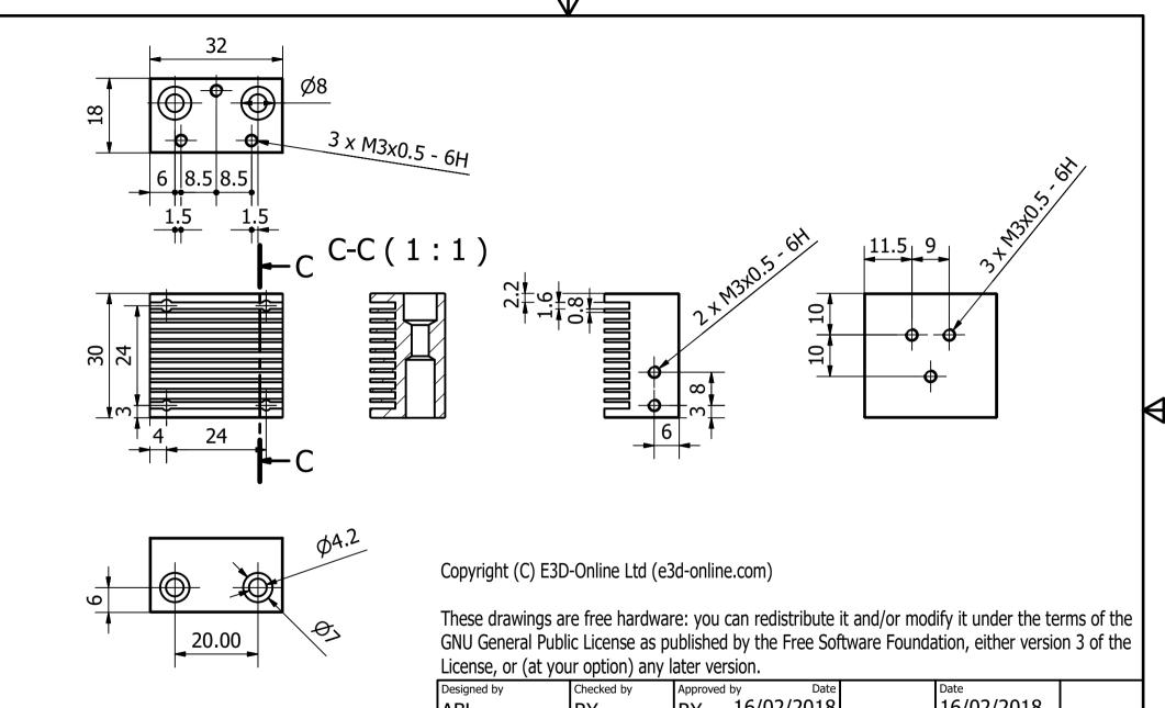
ALL DIMENSIONS IN MM MATERIAL: ALUMINIUM SCALE: 1:1
